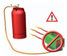
In order to avoid the gas cylinder(s) icing up, it is necessary to configure the gas supply in accordance with the unit connection value, the time in operation and the ambient temperature of the supply tank.
